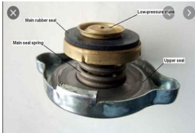
As the engine's coolant heats up, it expands, increasing pressure inside the closed coolant system. The radiator cap controls this expansion and provides constant pressure on the system.
