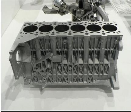
The crankcase is a metallic cover that holds together the crankshaft and all its attachments. It is the largest cavity within an engine that protects the crankshaft, connecting rods, and other components from foreign objects. Automotive crankcases are filled with air and oil, while Magnesium, cast iron, Aluminum and alloys are some materials used to make crankcases.
