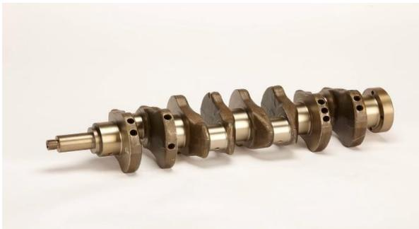
The crankshaft is a device which converts the up and down movement of the piston into rotary motion. This shaft is presented at the bottom of the engine and its main function is to rotate pistons in a circular motion. The crankshaft is further connected to the flywheel, clutch, and main shaft of the transmission, torque converter and belt pulley.
