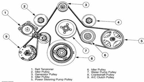
Engine belts are the bands made of flexible material used for connecting or joining two rotating shafts or pulleys together. These belts work in coordination with wheels and axles for transferring energy. When the wheels or shafts are positioned at extremely different angles, then the engine belts have the ability to change the direction of force. Engine pulley is a type of machine or wheel having either a broad rim or groomed rim attached to a rope or chain for lifting heavy objects.
