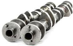
The camshaft is a type of rotating device or apparatus used in piston engines for propelling of operating poppet valves. The camshaft comprises of a series of cams that regulates the opening and closing of the valves in piston engines. The camshaft works with the help of a belt, chain and gears.
